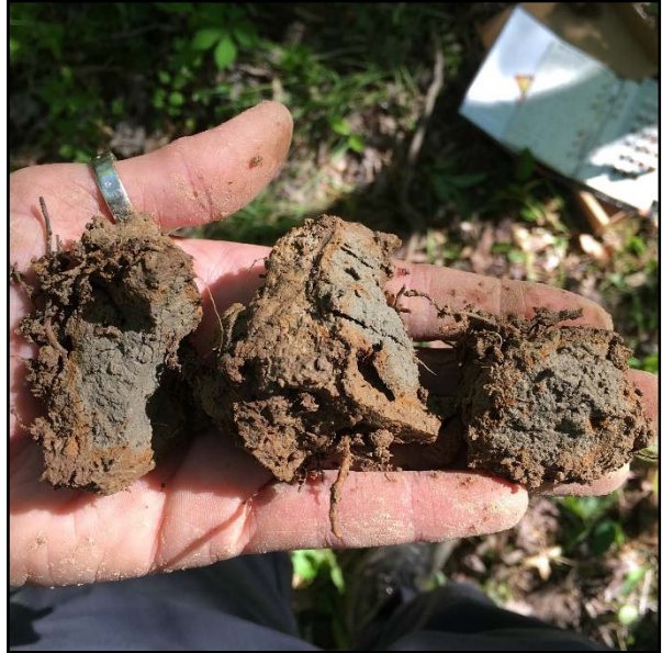
Photo 2: Soil sample showing depleted matrix and redox concentrations
